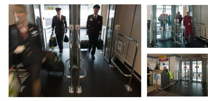
This record FlipFlow WIDE extended is installed at Glasgow International Airport. The units can be operated singly and so not used when not needed. The FlipFlow system allows safe and secure passage of persons into or from areas where security is a priority and a controlled flow of people is required.
