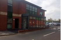
This refurbishment was at Veolia owned, Bolingbroke House in Battle field Enterprise Park in Shrewsbury. The refurbishment consisted of external curtain walling and external swing door (record's D 127 INVERSE) and internally an entrance of double sided Fine Frame sliding doors (record's STA 20 Fine frame)
